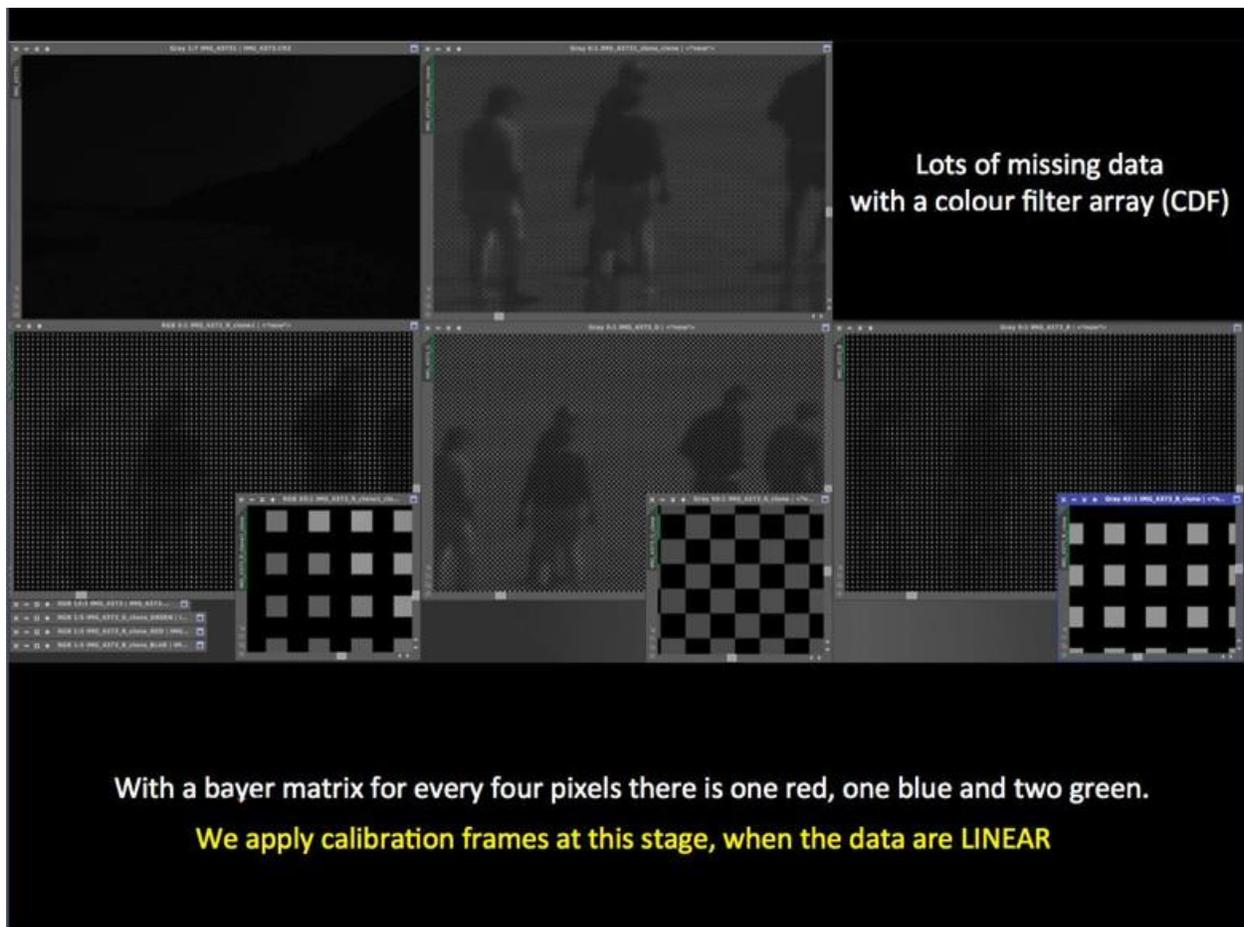
The top image is the combined RGB. The lower three are the RGB channels. They look somewhat “blocky”. If we zoom in further then we can see missing data. In the red channel there is one grey block for every three black and same with the blue channel. On the green channel there are two grey blocks and two black blocks. This corresponds to the Bayer Filter Array where there is one red, one blue and two green filters in every block of 4. So each channel has missing data.
